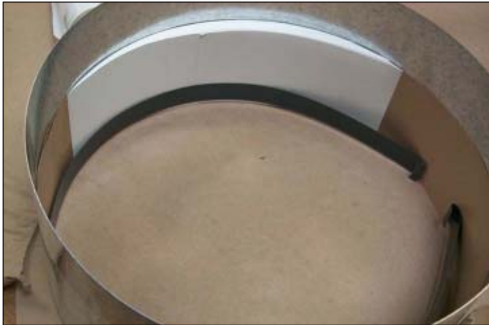
Figure K-6. Placement of Leaflets in Packing Ring
